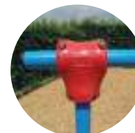
Vandalism resistant synthetic connection clamps. Metal parts are treated against corrosion and powdercoated with polyester.
